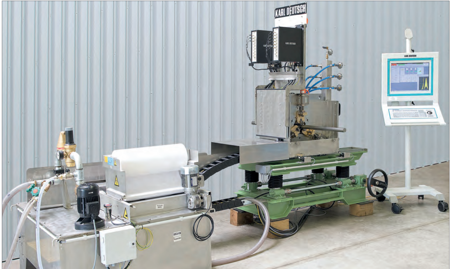
Bar testing system with water filter unit, test table and operator panel
