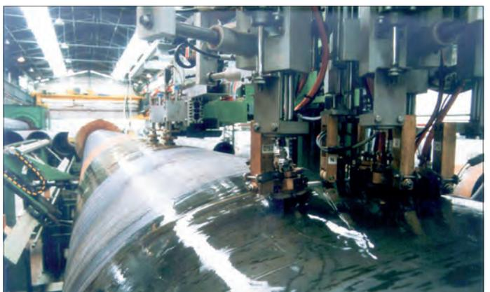
The pipe body can also be tested after welding (instead of testing the strip). The number of probes is chosen according to the required surface coverage and the welding speed. The coverage can be further increased with an oscillating probe movement.
