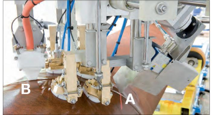
Six ultrasonic probes follow the weld crown which is monitored by a laser-optical seam tracker (A). The distance of the longitudinal probes with respect to the weld (skip distance) can be comfortably adjusted. The on-bead transverse probes are mounted into one common probe holder (B).
