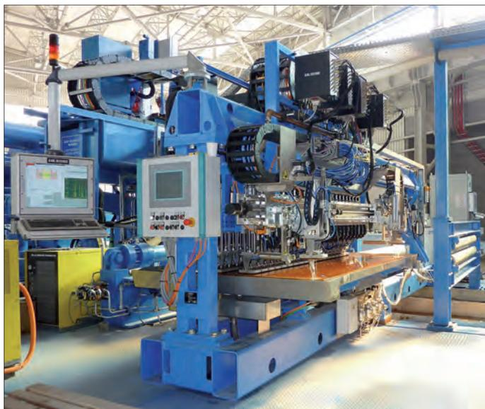
A strip test machine consists of a test bridge which is twice as wide as the steel strip width. The probe holders can be moved between test position (online) and calibration position (offline, see picture). For further details see our brochure ECHOGRAPH-BAPS.
