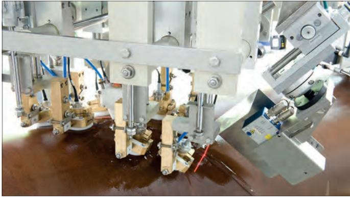
Close-up view of the weld crown monitoring by a laser optical tracking system
