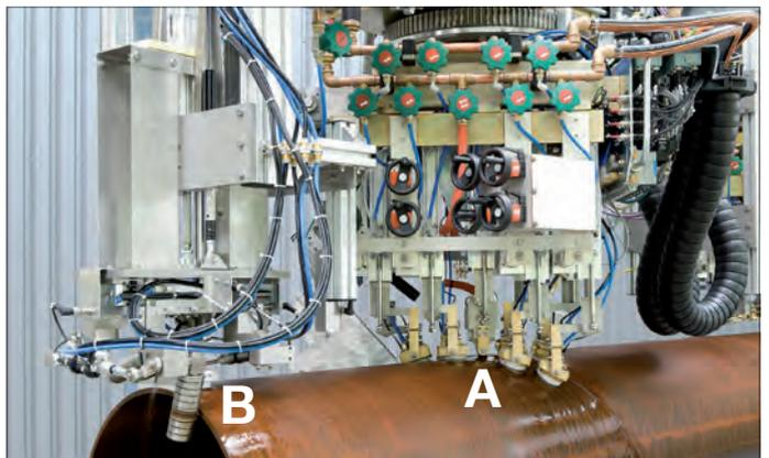
Due to the compact design of the probe holders, all required probes can be mounted into one test frame (A). The separate pipe end probe holder is seen on the left side (B).
