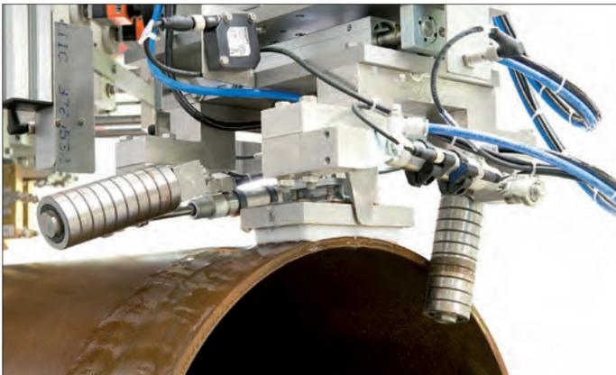
The pipe end testing uses a paintbrush probe with a 50 mm test track. Perfect guidance along the pipe end is achieved by a set of steel rollers. The same probe holder is used for both pipe ends (second set of steel rollers here in idle state).
