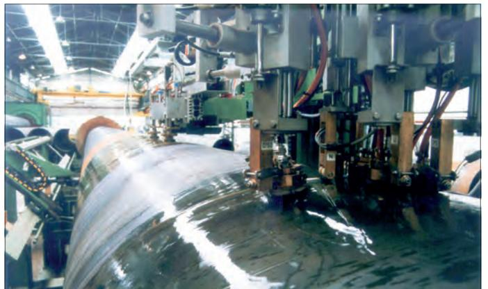
The pipe body can also be tested after welding (instead of testing the strip). The number of probes is chosen accordingly to the required surface coverage and the welding speed. The coverage can be further increased with an oscillating probe movement.
