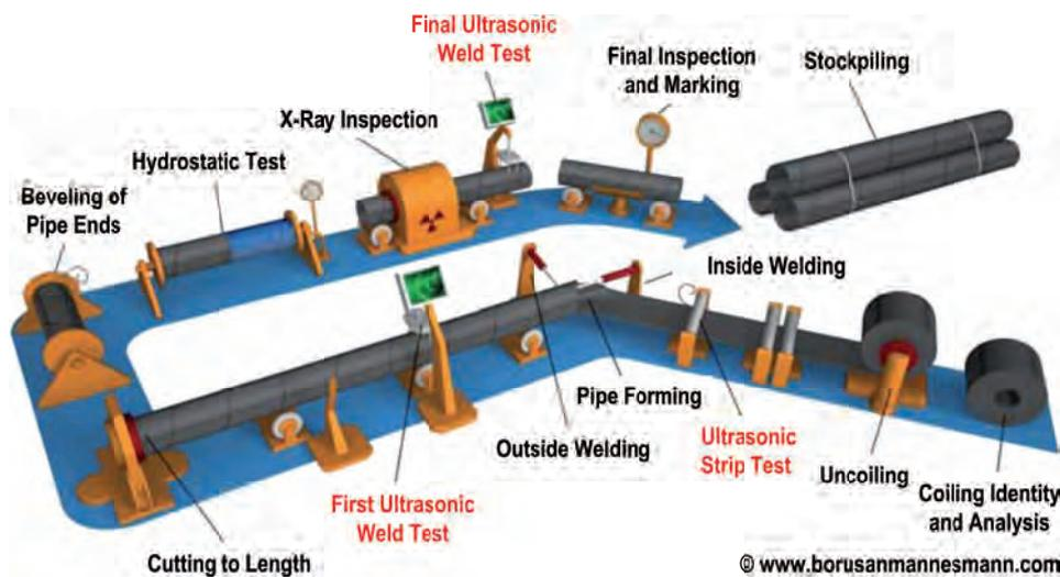
Production chart for helically (spirally) welded SAW-pipes (courtesy of Borusan Mannesmann Turkey): After uncoiling the steel strip, an ultrasonic strip test is executed. Then the pipe is formed and welded, followed by an on-line ultrasonic weld test. At the end of the line, the pipes are cut to their final length, then undergo a hydrostatic test, an X-ray inspection and the final ultrasonic weld test.
