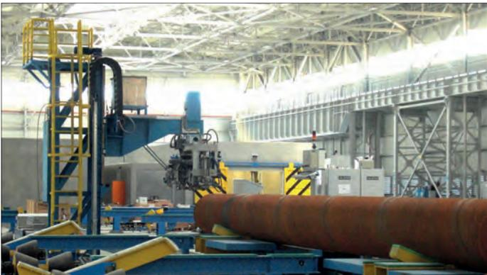
The pipe is handled by means of a pipe carriage. Linear and rotational feeding must be perfectly synchronised (picture courtesy of Borusan Mannesmann Turkey).
