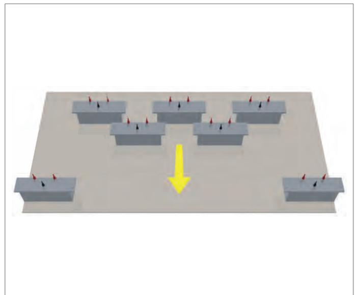
Testing of the flat metal sheet before welding with 100% coverage: The strip centre is covered by overlapping probes in two rows. Separate probe holders are used for the strip edges. They are guided along the edges by steel rollers.
