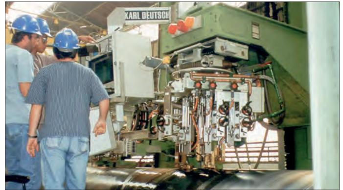
The weld testing mechanics is mounted to a height adjustable boom. Due to the large pipe diameter range, an operator's platform is often required.
