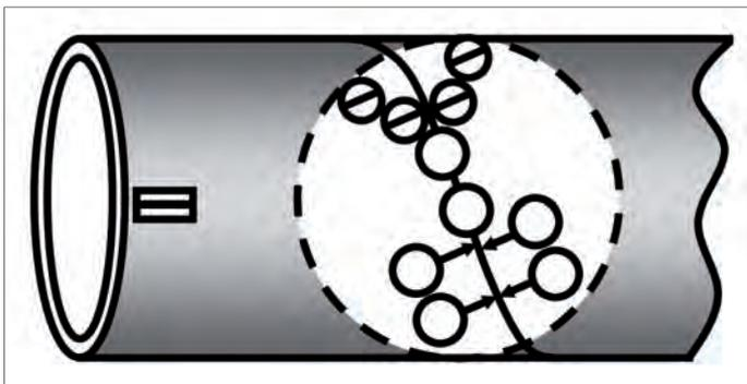
Schematic drawing of the probe configuration for online ultrasonic weld testing with 6 angle beam incidences for longitudinal and transverse defects and 4 straight beam incidences for detection of laminations within the pipe body and the heat-affected zones beside the weld.
