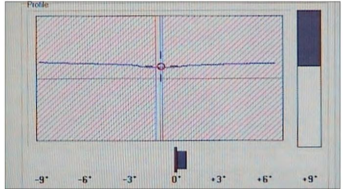
The result of the seam tracking system is always visible on the screen of the operating panel. Here, the probe pairs are perfectly centred with respect to the weld.
