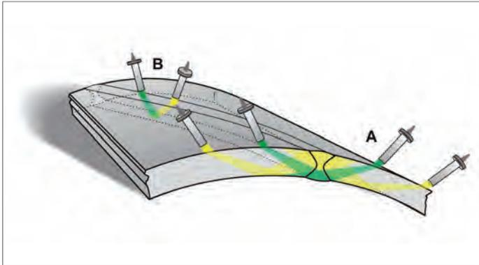
Online ultrasonic weld testing with six probes: A) two probes for external longitudinal defects, two probes for internal longitudinal defects; B) two on-bead probes for transverse defects.
