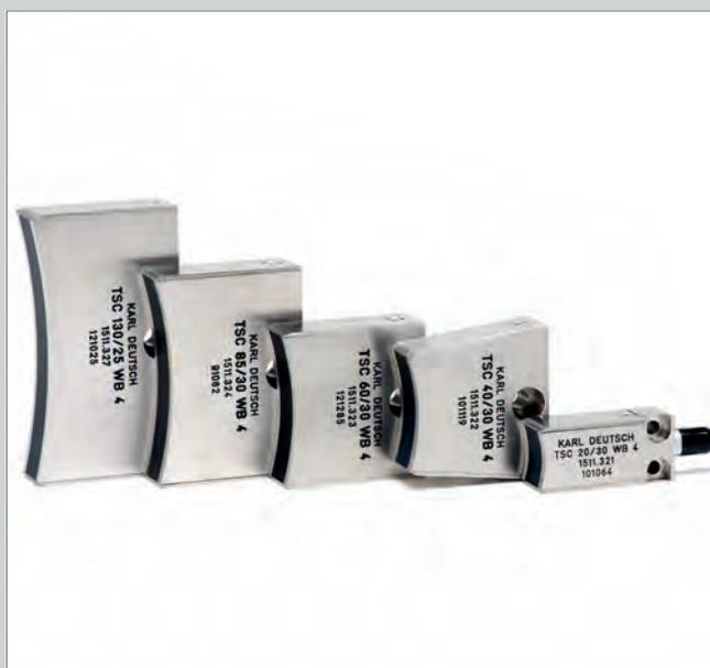
Special line-focused probes for angular incidence in different sizes to test the respective bar diameters: Each probe covers 30 degrees of the bar surface – independently from the bar diameter.
