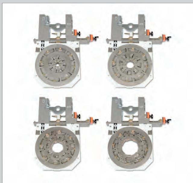
Test cassette with ring of ultrasonic probes: Angle beam probes are used to detect surface defects while straight beam probes are used to detect core defects. The testing angle of all angle beam probes is centrally adjusted by the spindle and the orange dial.
