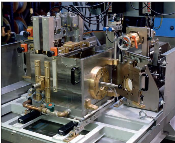
System calibration by means of short bar carrying artificial defects. The bar is rotated so the defect will pass each ultrasonic probe. Afterwards, the automated sensitivity adjustment equalizes the sensitivity of all probes. For the calibration process, the test chamber is moved into calibration position (offline).
